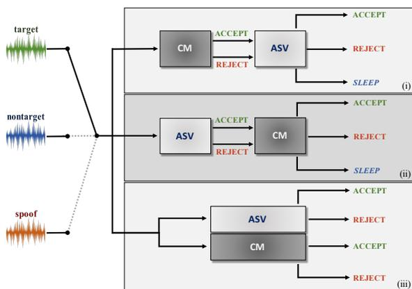
Figure 1: This work addresses performance assessment of a combined system consisting of an *automatic speaker verification* (ASV) module and a ‘plug-and-play’ *spoofing countermeasure* (CM) that are combined either (i) CM followed by ASV, (ii) ASV followed by CM, or (iii) in parallel. The combined system is subjected to benchmarking using speech utterances from three different types of users: targets, nontargets and attackers.
